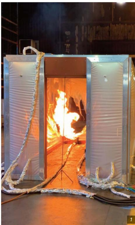
Figure 1. Flame after increase to 300kW.
