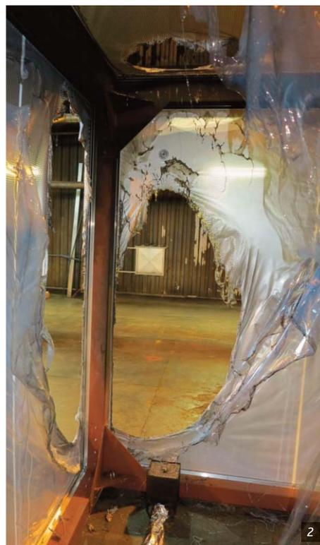
Figure 2. After the test holes of 1.5m<sup>2</sup> were formed in the façade foil cushions and a hole of 0.5m<sup>2</sup> was formed in the upper left corner of the roof cushion.
