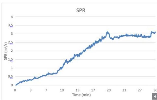
Figure 4. Smoke production rate during test including burner.
